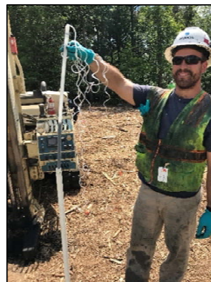
Photo 18: Bailed sample of groundwater from PZ-3 showing PlumeStop in sample.
