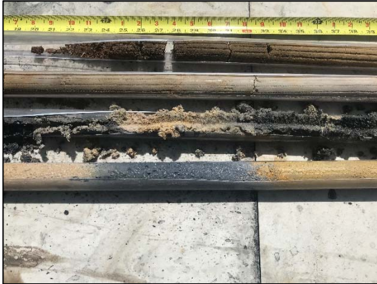
Photo 7: Post-application boring DV-1b showing concentrated PlumeStop in a banding pattern.
