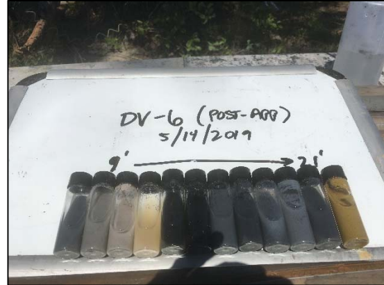
Photo 14: Core sediments demonstrating significant influence from 13-20 ft bgs.
