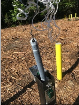
Photo 19: PlumeStop in bailed sample from one of the permanent monitoring wells in the area.
