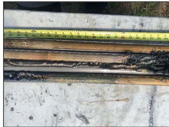
Photo 10: Post-application cores of DV-2b denoting PlumeStop concentration at depth.
