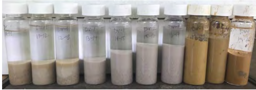
Figure 2. DV-1 soil settling tubes from 10 ft bgs (far left) to 20 ft bgs (far right) depicting the abrupt change from light tan sand (10-13 ft bgs) to light gray silty sand (13-17 ft bgs) to orange-brown clay beginning at 16.3 ft bgs. Complete boring log located in Appendix B: Soil Boring Logs.
