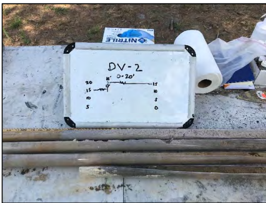
Photo 9: Pre-application soil boring DV-2.
